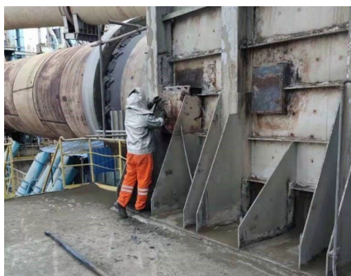
Hydrochloric acid bottles are incinerated in a preheater
